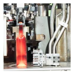
Emhart Glass universal conveyor supports the FlexPusher with special designed wind boxes and dead plates. New machines with FlexPusher will always delivered with the Universal Conveyor. Upgrades of existing machines with the FlexPusher also require the Universal conveyor. This makes such conversions quicker and reduces the risk of unforeseeable interference and ensures a low number of interfaces which need to be checked.
