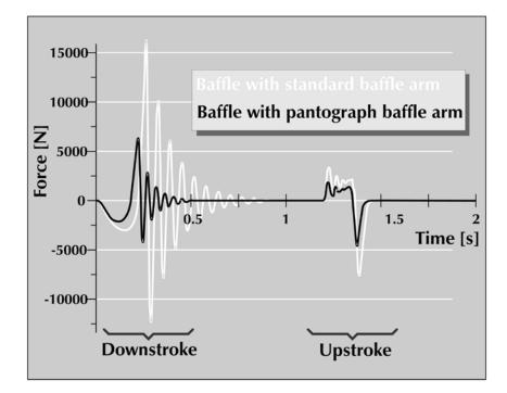
Compared with nonpantograph baffle applications, the curve for the baffle with the pantograph arm shows that there is approximately 60% less force acting on the entire unit. This is due to the reduced mass moment of inertia on the pantograph baffle application.
